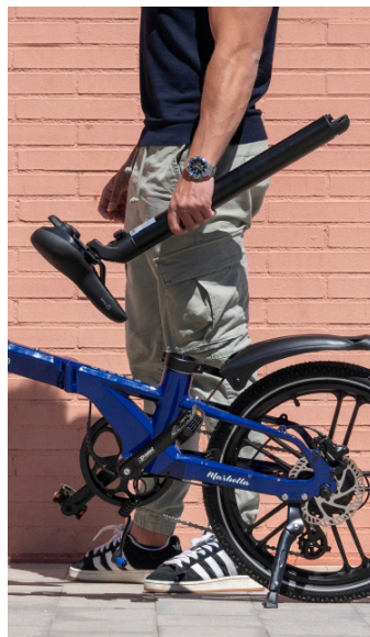
battery integrated into the seat post
